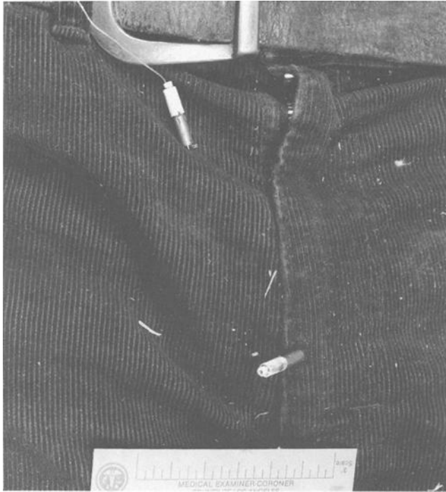
FIG. 3—Taser barbs imbedded in trousers. The 1 to 1½-in. (25.4 to 38-mm) spark makes the Taser effective.
